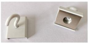
\*We test the holding force of magnetic assembly by attaching it on a 20mm thick steel sheet at room temperature and then pulling it slowly in vertical direction with the device that is sensitive enough to record the strength at the moment when magnetic assembly is separated from the steel sheet. This is to give you a reference where the actual holding force in real application could be different with the change of, for example, pulling direction, thickness of the surface etc.
