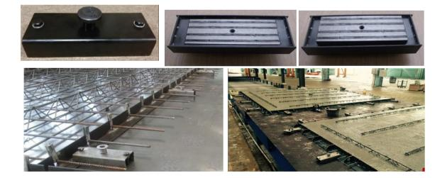
\*We test the holding force of magnetic assembly by attaching it on a 20mm thick steel sheet at room temperature and then pulling it slowly in vertical direction with the device that is sensitive enough to record the strength at the moment when magnetic assembly is separated from the steel sheet. This is to give you a reference where the actual holding force in real application could be different with the change of, for example, pulling direction, thickness of the surface etc.
