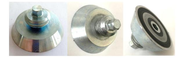
\*We test the holding force of magnetic assembly by attaching it on a 20mm thick steel sheet at room temperature and then pulling it slowly in vertical direction with the device that is sensitive enough to record the strength at the moment when magnetic assembly is separated from the steel sheet. This is to give you a reference where the actual holding force in real application could be different with the change of, for example, pulling direction, thickness of the surface etc.
