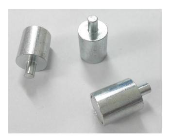
\*We test the holding force of magnetic assembly by attaching it on a 20mm thick steel sheet at room temperature and then pulling it slowly in vertical direction with the device that is sensitive enough to record the strength at the moment when magnetic assembly is separated from the steel sheet. This is to give you a reference where the actual holding force in real application could be different with the change of, for example, pulling direction, thickness of the surface etc.
