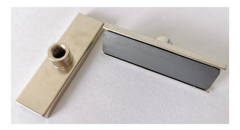
\*We test the holding force of magnetic assembly by attaching it on a 20mm thick steel sheet at room temperature and then pulling it slowly in vertical direction with the device that is sensitive enough to record the strength at the moment when magnetic assembly is separated from the steel sheet. This is to give you a reference where the actual holding force in real application could be different with the change of, for example, pulling direction, thickness of the surface etc.
